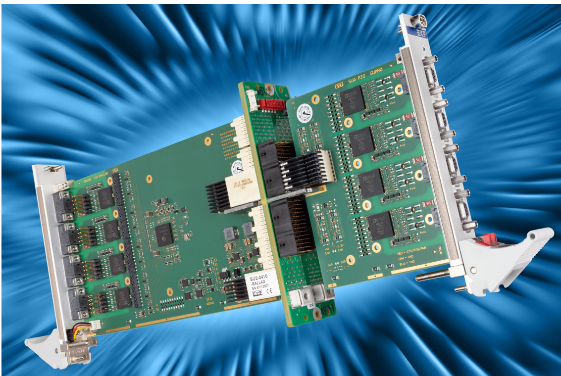
SUA-RIO w. SU2-BALLAD (Eight Port 4HP Isolated RS-232 Solution)
